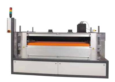
PP board made of blended PP co-polymer has one major disadvantage - low surface energy, resulting in poor surface adhesion for water-based adhesives and inks. Corona treatment systems by Tantec significantly increase surface energy and improve adhesion.
