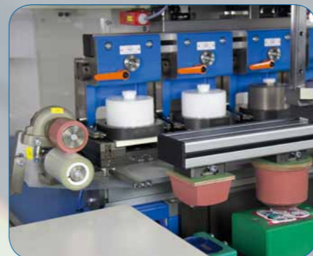
TSM 60/90 universal multiple colour kit Solo with “ink residue pick-up system”
