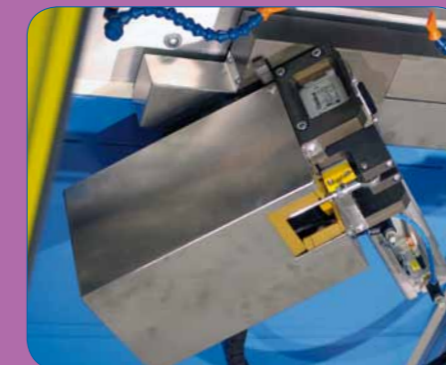
Rotary device autom. positions workpieces for double-sided pad printing process.
