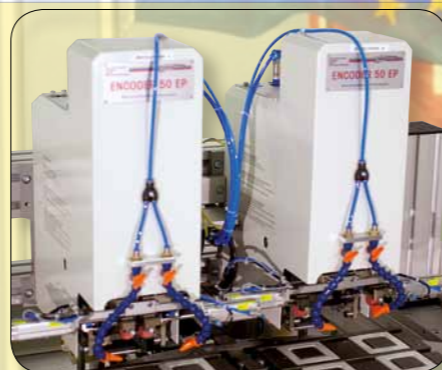
Automation with pad ventilation for light switch frames
