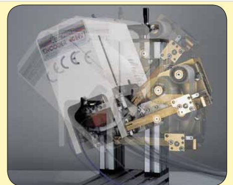
ENCODER /1 – Integration position between 90°–180° with ink residue pick-up system
