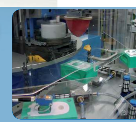
CONCENTRA 90-4 with rotary index table, jig with vacuum support
