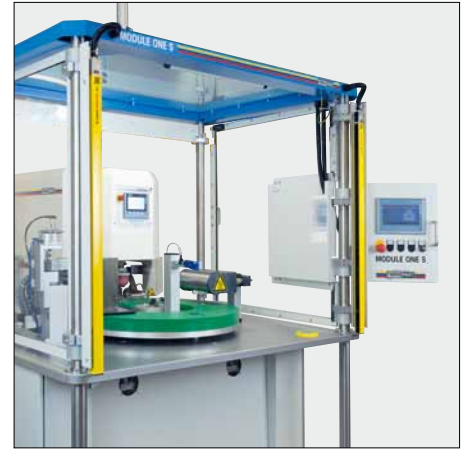
Ergonomic: User-friendly, rotating operator panel (integrated in side door)
