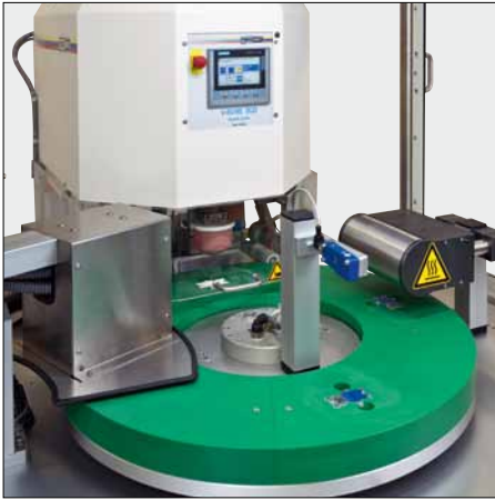
Multifunction jig surrounded by pad printing machine and components (Illustration: Corona pre-treatment, parts detection, infrared drying)
