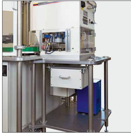
Assembly of satellite to rear side of machine with easy access to the printing units (picture with optional drawer)
