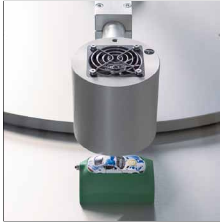
Component intermediate-drying – light surface drying of the pad printing ink for faster continuous printing
