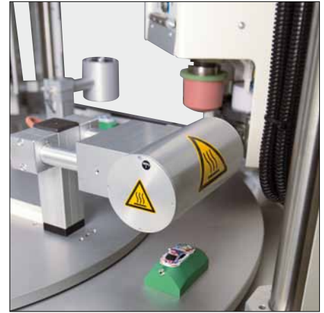
Component infrared-drying – shortens the drying time of the pad printing ink
