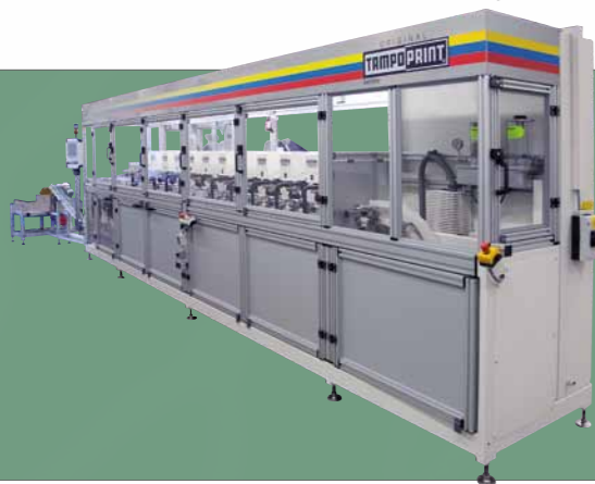
Reference Toy industry: Fully automatic 12-colour pad printing system Performance: 24.000 printing parts/h
