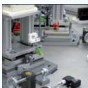
x/y plate cross table with swivel device
