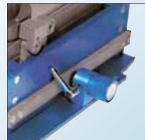
Detail: x-y adjustment by means of micrometer screw
