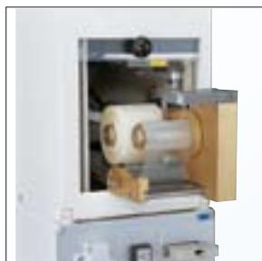
Ink residue pick-up system (tampon cleaning)
