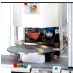
„T2“ index table to fit the workpieces
