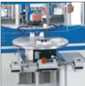
Index table „T2“ to fit the workpieces
