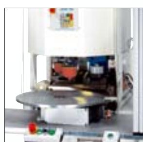
„T2“ index table to fit the workpieces
