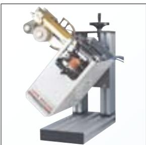
Aluminium stand / ink residue pick-up system right
