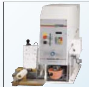
Ink residue pick-up system attached on the left
