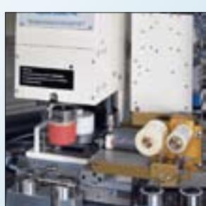
Ink residue pick-up system attached on the right
