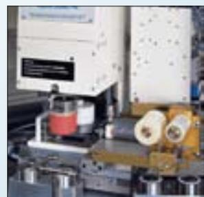
Ink residue pick-up system attached on the right
