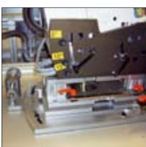
Cross table with inclination adjustment
