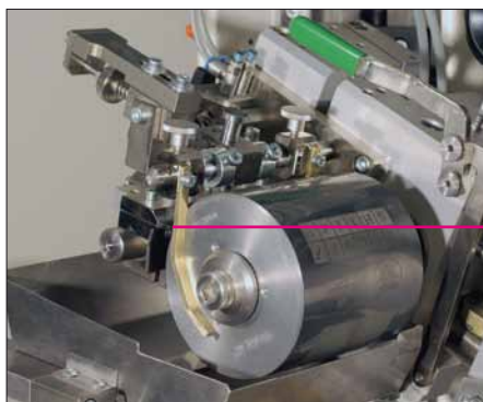
Fig.: "Hightech ceramic cliché cylinder" installed in rotary tampon printing unit
