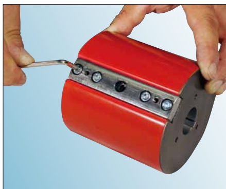
Fig.: Magnet-screen clamping cliché "R" is mounted to the clamping cylinder
