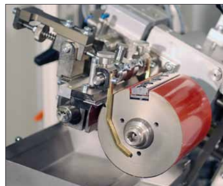
Fig.: Clamping cylinder mounted in rotary tampon printing unit
