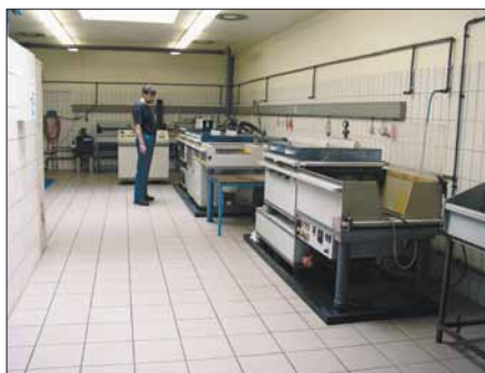
Etched, using automatic cliché etching lines
