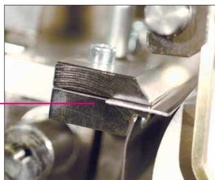
Fig.: Rotary printing doctor blade in rotary tampon printing unit
